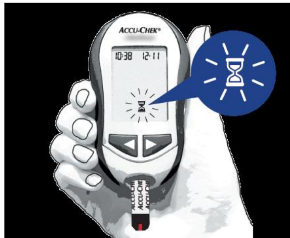
Figure 6.9 Test strip has required blood volume
