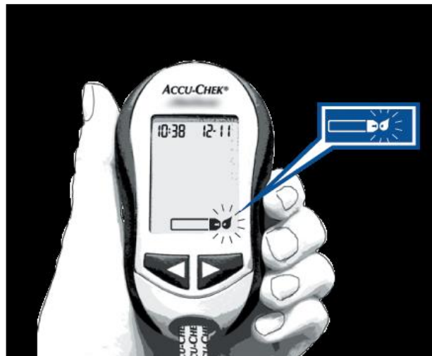
Figure 6.6 'Apply Sample' symbols on glucometer display
